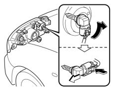
3. Install the new socket and bulb assembly in the reverse order of removal.
